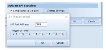
You can specify the pin(s) on which the signal is send. This signal is stored in the BRAIN PRODUCTS specific marker file.
